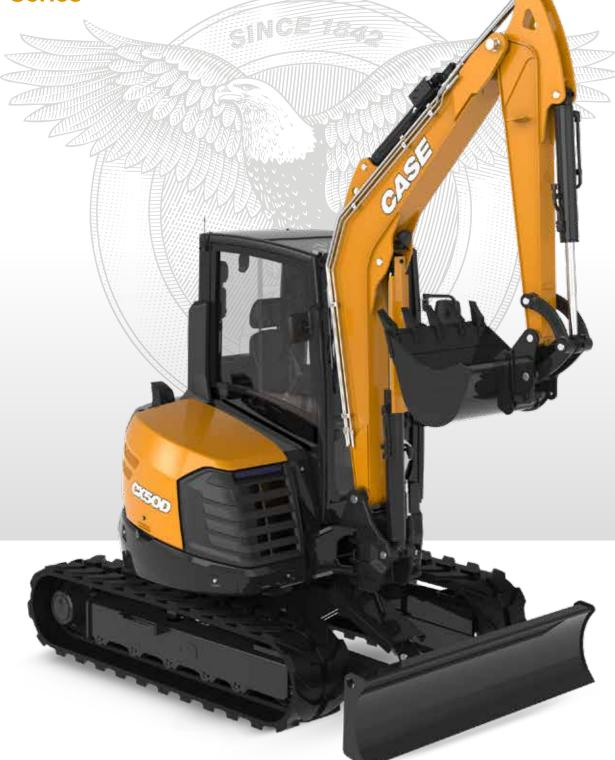
Engine V2403-CR-T Engine power 42.6 kW - 57.9 hp Operating weight 4800 kg
