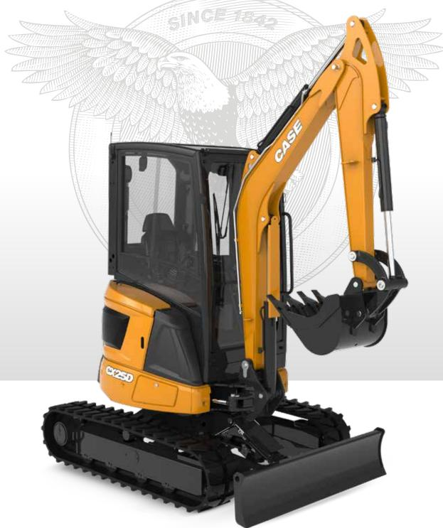
Engine 3TNV76 Engine power 15.5 kW - 21.1 hp Operating weight with canopy 2410 kg Operating weight with cab 2540 kg
