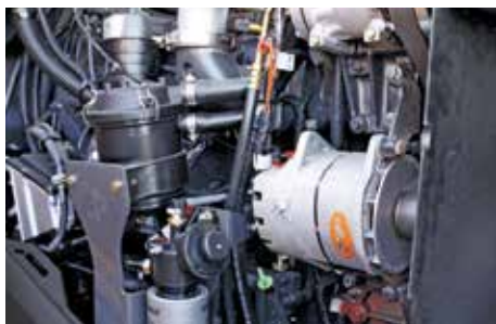
Fuel filter and engine oil service points are easily accessible from both sides while the others filters are behind the right stairs
