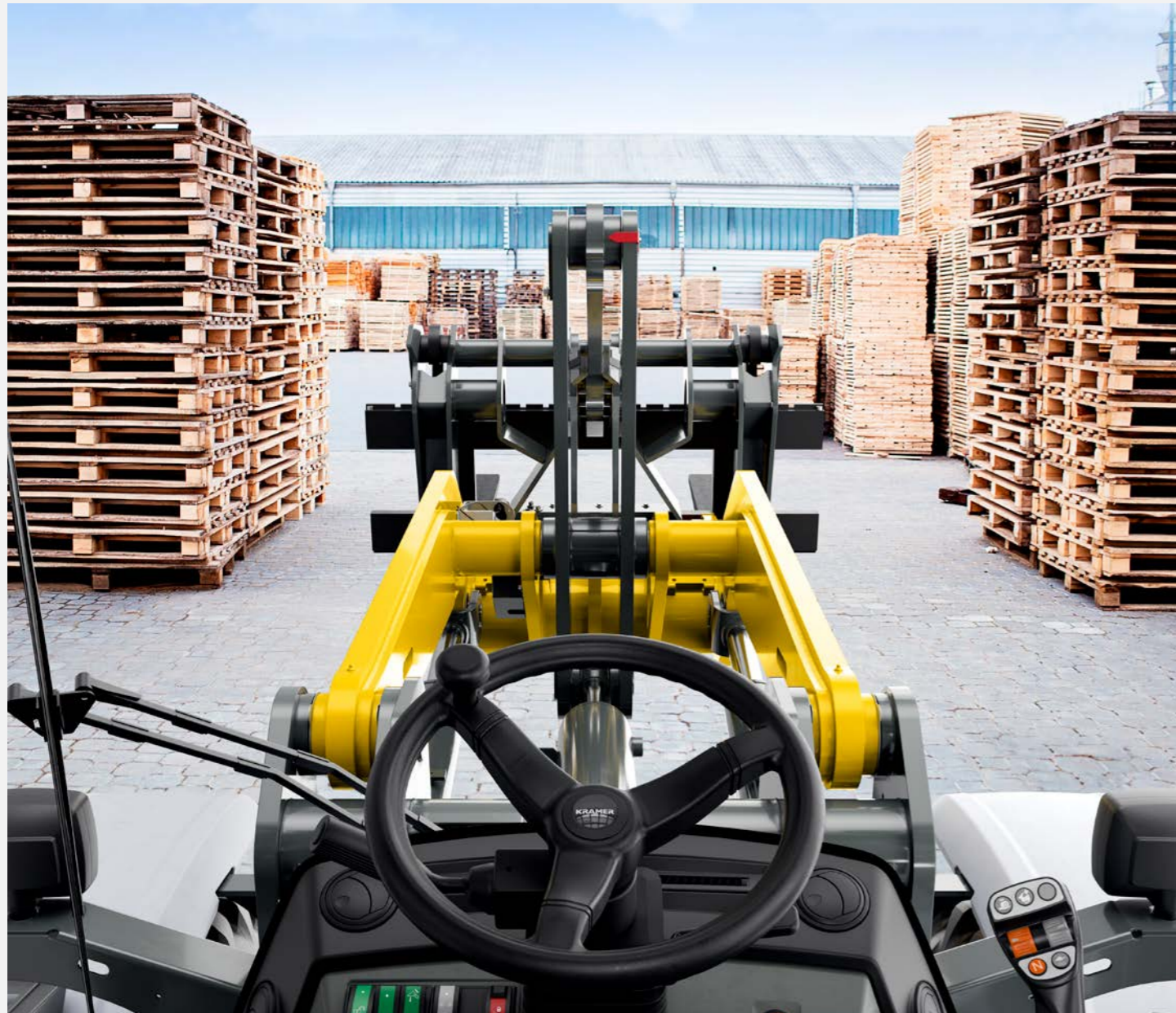
Excellent all-round visibility: narrow cabin struts and panoramic glazing offer an optimal view on all sides.
