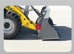
The Kramer quick-hitch system: Drive up to the attachment. Hydraulically mount the attachment from the seat and with a clear line of sight. Control the process with the touch slide on the joystick.
