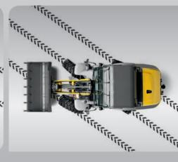
Crab steering is ideal for parallel movement and manoeuvring in confined spaces, e.g. when clearing industrial buildings.
