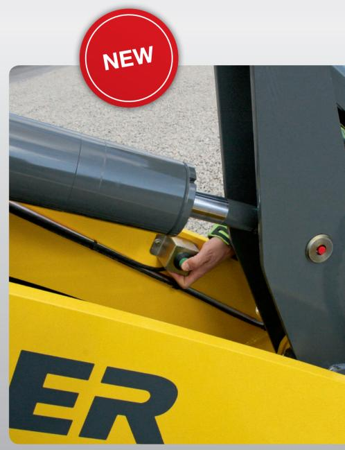
Pressure release in the 3rd control circuit for easy connecting and disconnecting of attachments with hydraulically activated auxiliary functions.
