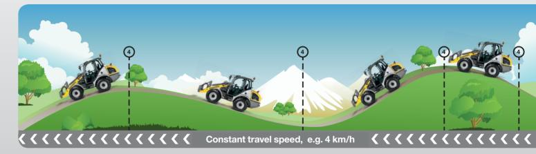
When using attachments that, for example, are operated at a constant high RPM, but at the same time with a very low travel speed (e.g. a sweeper), the specifications can be realised simultaneously by the creep speed controller in conjunction with the hand throttle.
