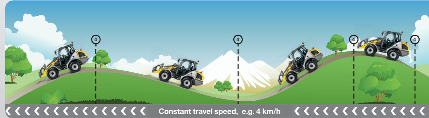
When using attachments that, for example, are operated at a constant high RPM, but at the same time with a very low travel speed (e.g. a sweeper), the specifications can be realised simultaneously by the creep speed controller in conjunction with the hand throttle.
