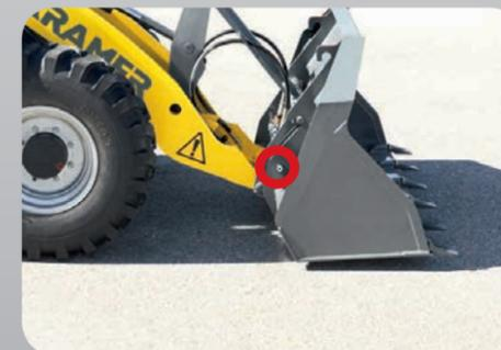
**The Kramer quick-hitch system:** Drive up to the attachment. Hydraulically mount the attachment from the seat and with a clear line of sight. Control the process with the touch slide on the joystick.
