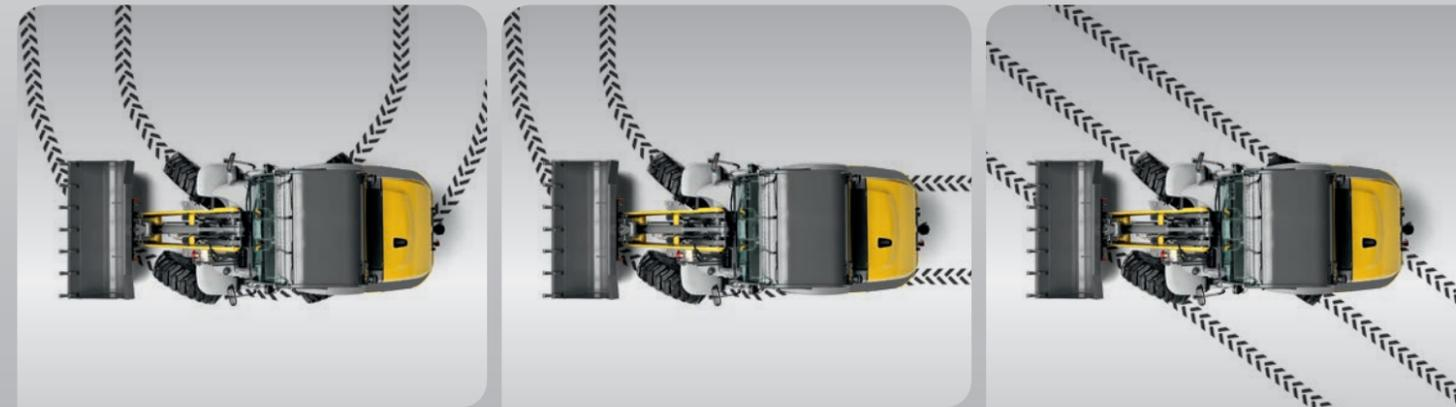
The **all-wheel steering** is particularly manoeuvrable due to its 2x40-degree steering angle.
