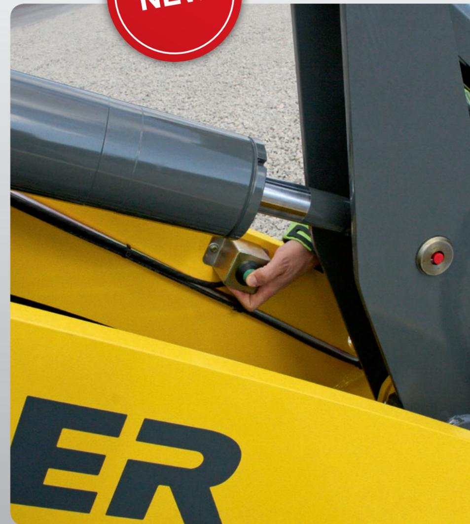
**Pressure release in the 3rd control circuit** for easy connecting and disconnecting of attachments with hydraulically activated auxiliary functions.
