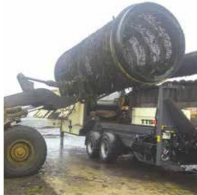
Easily replaced 5.5m (18') x 2m (6'7") punch plate drum which is compatible with the Doppstadt SM620 and Neuenhauser 6020
