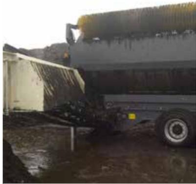
Double sided unrestricted drum access via two large swing out doors allows for easy maintenance and cleaning
