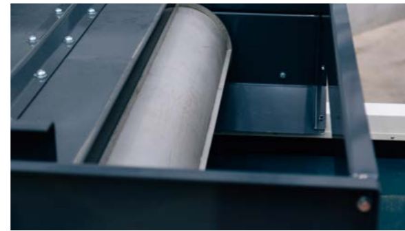
Variable speed 2m (6' 7") wide high strength neodymium radial pole drum for optimal ferrous metal recovery
