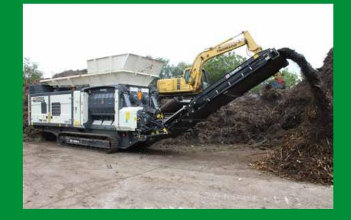
The TDS V20 screen system which is available in different sizes, comes complete with an intelligent protection system, allowing a desired particle size to be produced, whilst still being able to cope with foreign objects.
