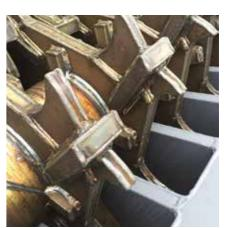
Shaft cutting elements are a fully welded structure with hard-faced edges giving ultimate strength in difficult applications
