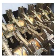
Robust German designed shredding chamber Independently driven shafts give excellent shredding performance in even the most challenging of applications
