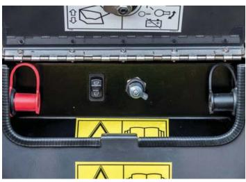
Hood opening and battery on/off switches. In case of flat battery, hood can be opened externally with Remote jump start
